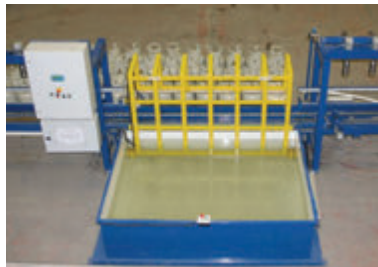
Pneumatic Leakage Testing Unit
